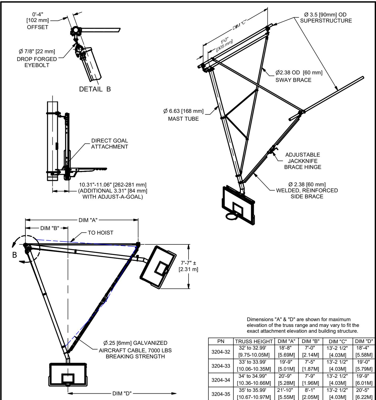
Dimensions "A" & "D" are shown for maximum elevation of the truss range and may vary to fit the exact attachment elevation and building structure.
