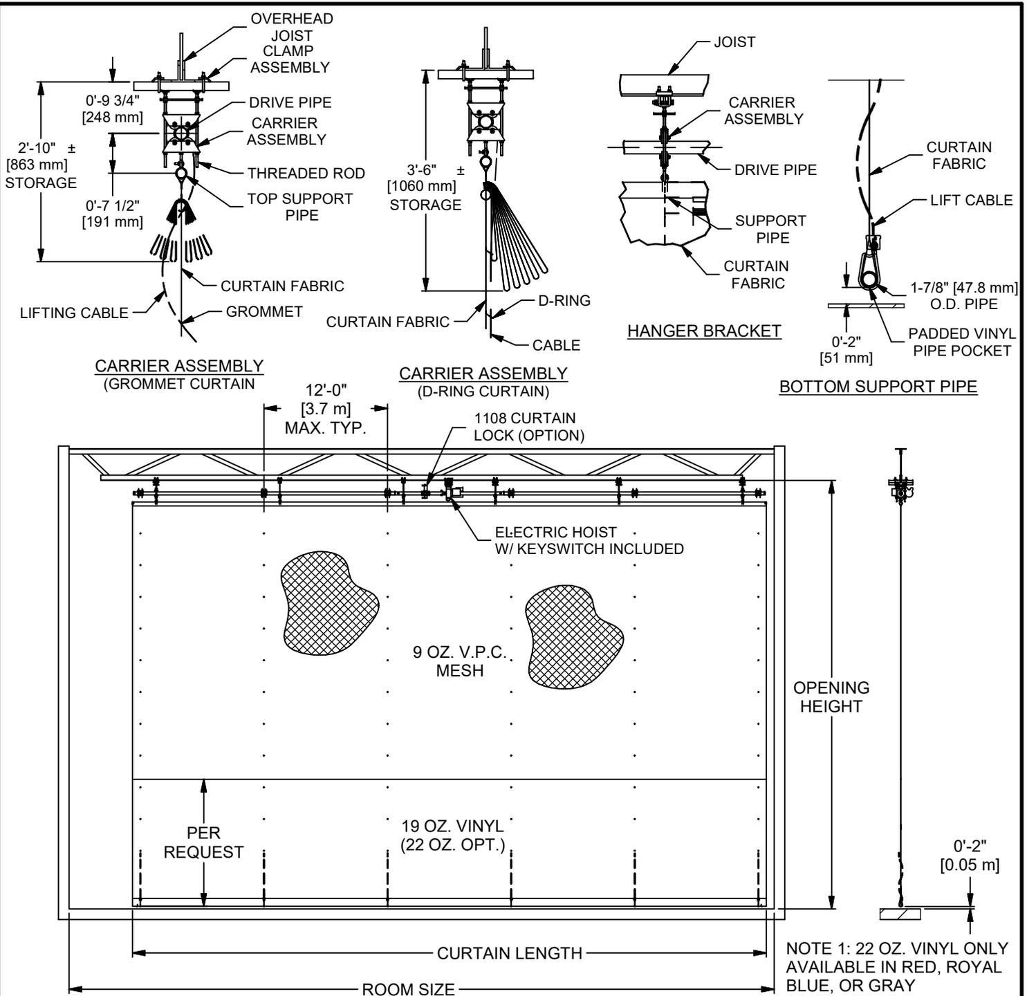
STANDARD MOTOR IS 3/4 HP, 120 VOLT, 60 HZ, SINGLE PHASE WITH KEY SWITCH & RECEPTACLE. MOTORS FOR OTHER POWER REQUIREMENTS ARE AVAILABLE. SEE SPECIFIC MOTOR SPECIFICATION DRAWINGS.
