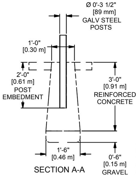
CONCRETE FOUNDATION SUPPLIED BY OTHERS. FOUNDATION SIZE SHOWN IS MINIMUM AND SHOULD BE REVIEWED USING LOCAL WIND LOADS AND SOIL CONDITIONS.
