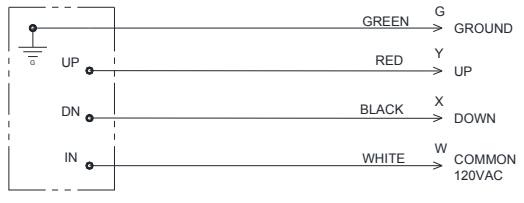
TSC1500 RELAY PANEL WITH TSC1500 / X / XL WIFI OPTION USED IN PLACE OF KEY SWITCH
