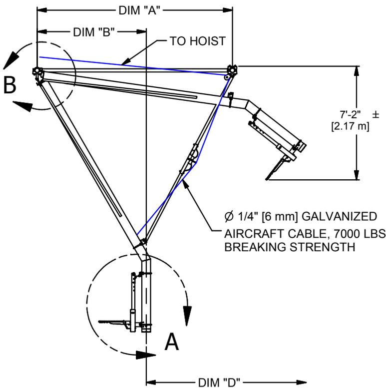
Dimensions "A" & "D" are shown for maximum elevation of the truss range and may vary to fit the exact attachment elevation and building structure.
