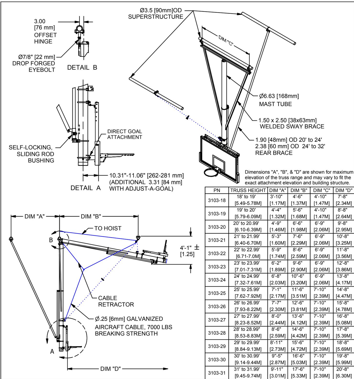
Dimensions "A", "B", & "D" are shown for maximum elevation of the truss range and may vary to fit the exact attachment elevation and building structure.
