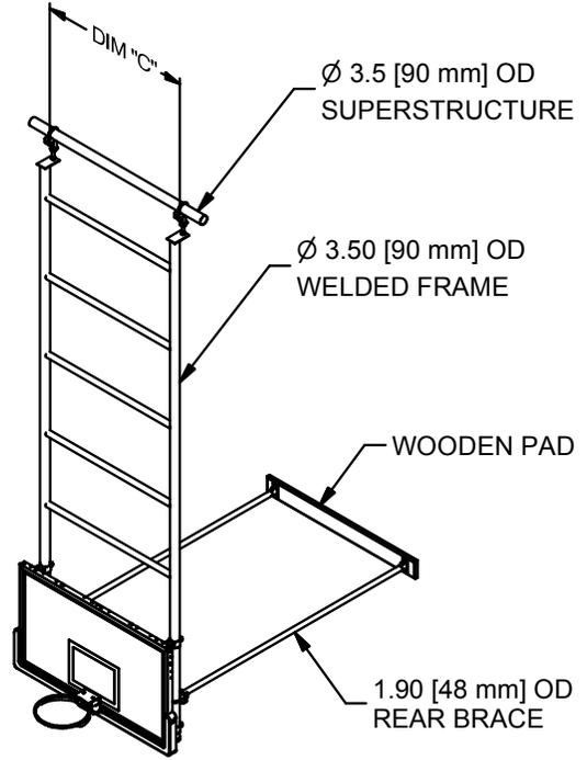
NOTE: DIM "C" IS 63" [1600 mm] WITH A RECTANGULAR BACKBOARD AND 35" [889 mm] WITH A FAN SHAPED BACKBOARD
