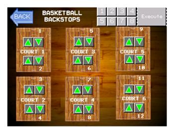
Once the operator releases the Execute button, the equipment will stop moving.
