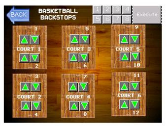
The red arrows indicate the direction the equipment will move when the Execute button is held down.
